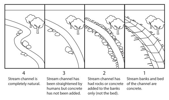
Use the diagram below to help you measure channel condition in the stream.
